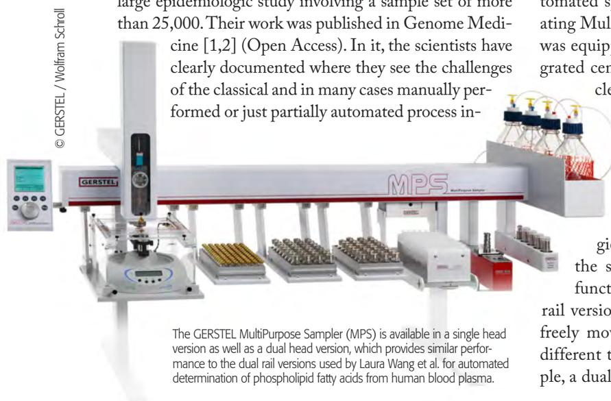
The GERSTEL MultiPurpose Sampler (MPS) is available in a single head version as well as a dual head version, which provides similar performance to the dual rail versions used by Laura Wang et al. for automated determination of phospholipid fatty acids from human blood plasma.
